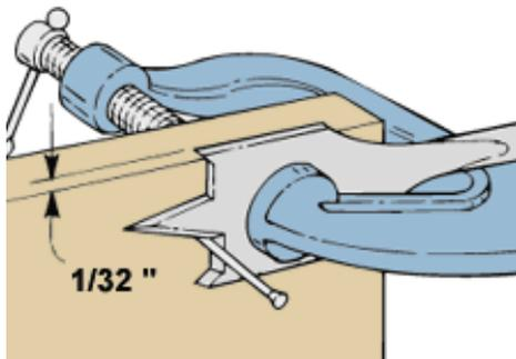
amount of material from each side. A handy way to do this is to use a nail and scrap block to position the bit, see drawing above. The nail positions the side of the bit 1/32"
