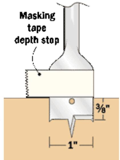
The second time around, I started with the counterbore. That way, you can use the centerpoint of the larger hole to center the bit when you drill the through hole.
