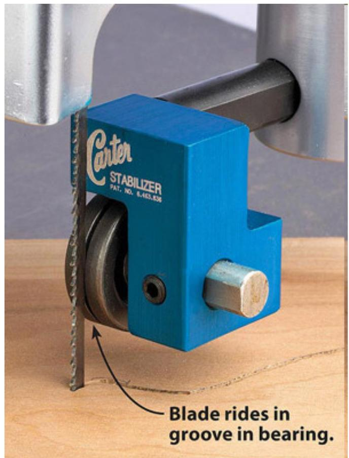
blade rides in a groove in the bearing's edge. The groove provides side-to-side support and the bearing reduces friction. Carter Products makes these as well but do not fit all models.
