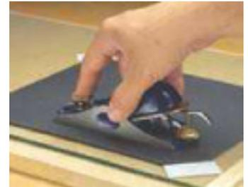
STEP TWO Then sand the sole on a sheet of 220- grit silicon carbide sandpaper that's taped to a piece of glass.
