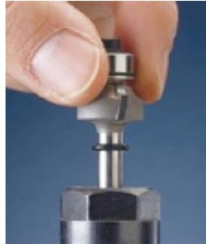
But it's hard to hold the bit and tighten the collet at the same time. So slip a common rubber O-ring around the shank of the bit, see photo. It holds the bit at the correct height. You can use this same trick for properly positioning the shank of a drill in your drill press. From ShopNotes.
