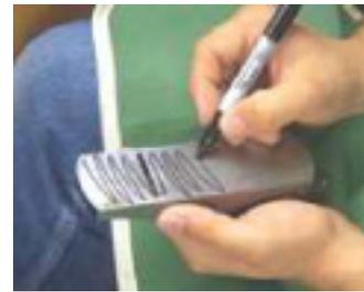
STEP ONE Using a permanent marker, draw a squiggly line across the sole of the plane.
