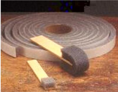
So you can make "instant" foam brushes by sticking pieces of self-adhesive foam weatherstripping on sticks made from scrap pieces of wood. For larger brushes, wrap the weatherstripping around the end of the wooden stick.
