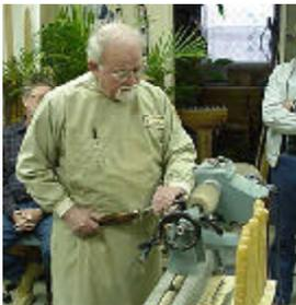
Bob first addressed lathe setup. Besides following the manufacturer's recommendations and safety advise, be certain you have adequate room in which to work and adequate light. A table to lay your tools and measuring equipment is also desirable. It is also very important to provide yourself eye and face protection using a full face shield or at minimum, safety
