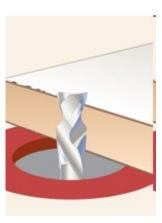
edge like a downcut bit, but rather to remove the chips created in a deep plunge cut. That makes it ideal for plowing out a deep mortise in solid stock. Tear-out caused by the upward shearing will be hidden by the tenoned workpiece.
