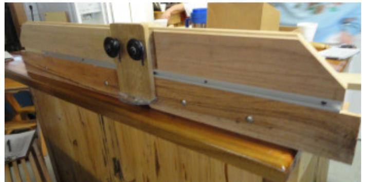
as a hold-down on a tablesaw fence. Since the wood is cut cross-grain, plywood is the best answer.
