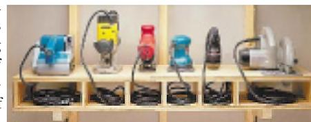
One last thing — not all tools will rest flat on the shelf. You can modify the top as needed by cutting slots or drilling holes for some of the tools. From *ShopNotes*.
