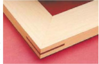
To cut the kerf for the spline, use a shop-made jig that straddles the rip fence on the table saw, as shown in the drawing right.
