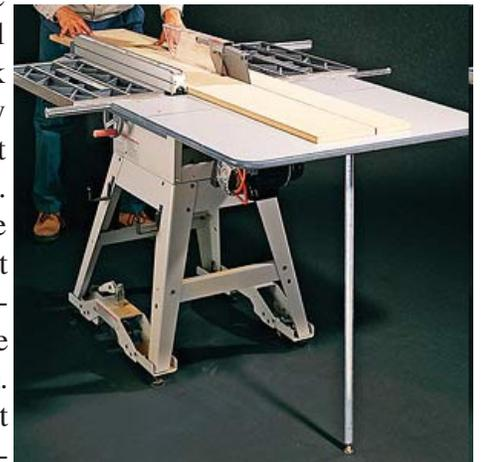
A permanent outfeed table isn't practical in a small shop: You just can't dedicate that much real estate to it. The fold-down outfeed table, extends 3' of support beyond the blade, yet adds only a few inches of depth to the back of the saw when stowed. And it's always ready, even on a mobile-base-equipped saw. (You'll find plans for a good outfeed table at [woodmagazine.com/outfeedtable](http://woodmagazine.com/outfeedtable).) *Barry Humphus with help from the great folks at .Wood Magazine.*
