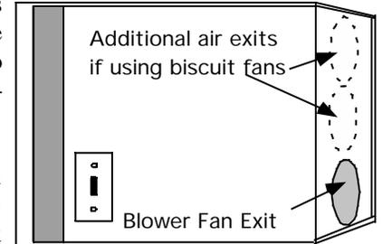
Where the air exits the box, cut a hole in the plywood large enough in diameter to accommodate your fans or blower. If you use biscuit fans, surface mount them on the inside of the rear piece over the exit holes. See the drawing above. A blower needs to be mounted such that it's venturi tube exits to an appropriately sized hole.
