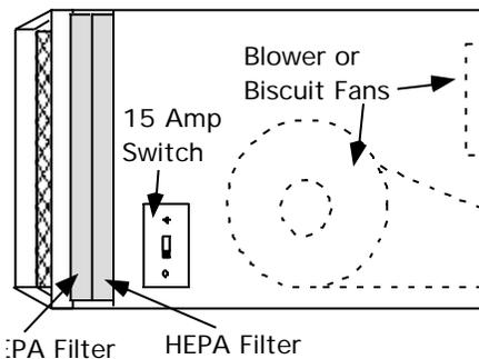
shop and large blower circulates the air at up to 20 times per hour under ideal conditions (door and windows closed).
