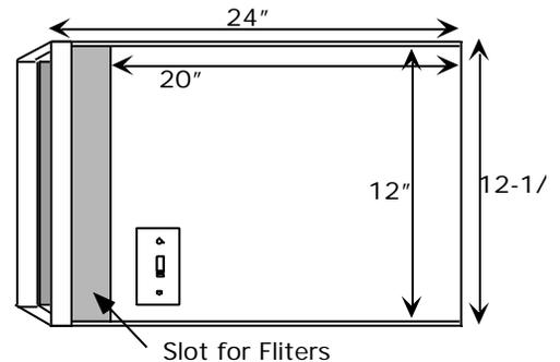
Position the air filter such that it provides a circulation of the shop. In other words, at one side of the shop. Mine is on a high shelf to one side and angled slightly into the room.
