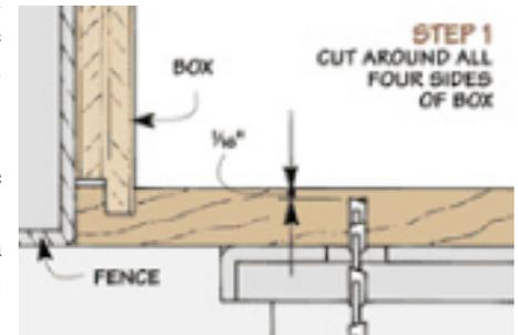
To avoid this, set the height of the saw blade so it's slightly less (1/16") than the thickness of the box, see Step 1. This leaves a thin membrane that holds the box together and keeps the kerf from pinching the saw blade.
