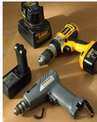
The earliest battery-powered drills in the 1970s were bulky and featured low-voltage batteries, but still seemed like a godsend because they had no power cord. Over the past 25 years manufacturers have boosted power significantly while cutting charge times and weight. They've also added keyless chucks and adjustable clutches, ergonomic designs, and other battery-powered tools, such as circular saws, reciprocating saws, jigsaws, and impact drivers.
