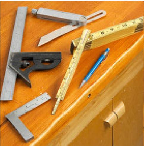
For longer dimensions, a 6' folding wooden rule provides more reliable accuracy than a retractable steel tape measure because there's no hook on one end that can get damaged and affect the accuracy. Get the kind with a sliding extension for dead-on measurement inside cases and boxes.
