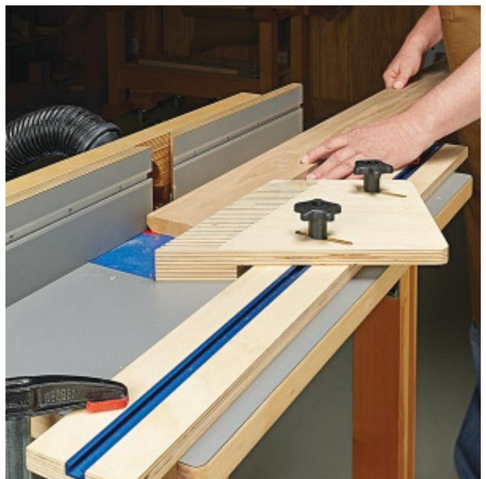
The featherboard system is easy to build. It consists of a plywood base with a section of T-track recessed in a groove cut in the surface of the base. The finger end of the featherboard has two layers. This allows the fingers to sit flush on the machine surface. Continues on Page 3 . . .
