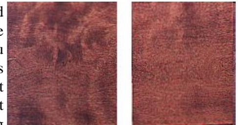
As shown in the photo above, gel stains help you achieve uniform coloration on these woods. Although you can buy "conditioners" specially made for sealing hard-to-stain woods prior to staining with thin-bodied stains, that combination did not give us as good a result as gel stains did.
