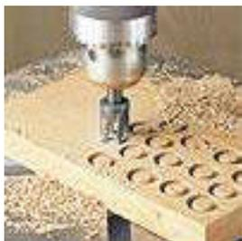
An easy way to get around this is to cut your own plugs. This way, you can cut a face grain plug that will absorb finish more easily. Another advantage is that you can use the scrap pieces remaining from a project to create an almost invisible plug, as shown in the photo. Or maybe you'd like to highlight the plug by using a type of wood that contrasts in color.
