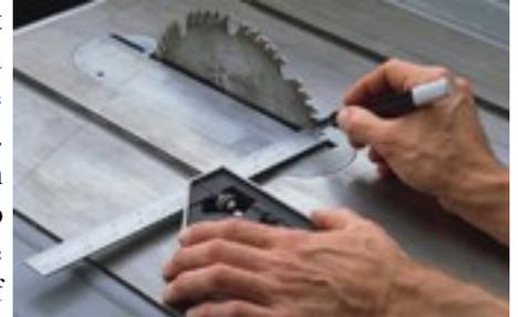
Next, slide the square and rotate the blade backward until the marked tooth aligns with the square. If the square just touches the side of the tooth, the slot and the blade are aligned. *Edited from woodworkingtips.com.*
