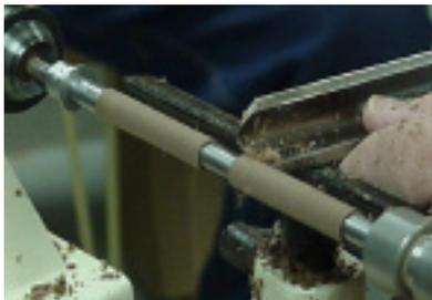
To turn the blanks, you need a pen mandrel (available from pen suppliers) mounted in your lathe's head stock. The mandrels come with standard Morse tapers and others. The mandrels come in different diameters depending on the kits you buy. The cost of the mandrels range from \$15 to \$28
