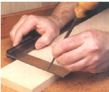
There are quite a few woodworkers who prefer a sharp awl to a pencil. The thin, tapered blades of awls make them particularly useful for reaching into tight quarters, such as when marking pins for dovetails. You can use one in lieu of a marking knife (bottom photo); just make sure to keep the point razor-sharp, as it will
