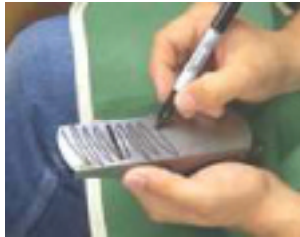
STEP ONE Using a permanent marker, draw a squiggly line across the sole of the plane.
