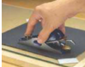
STEP TWO Then sand the sole on a sheet of 220- grit silicon carbide sandpaper that's taped to a piece of glass.
