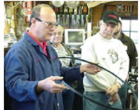
Hand saw blades can be sharpened in his shop as well. But Ed says that there is not a big demand for this any more. Still another machine does this in an automated way that sharpens and sets the teeth. He does not sharpen Japanese saw blades as these are typically edge hardened. That is, only the sawing edge is hardened so the sharpening process would take enough metal off the steel to go past the hardened part.
