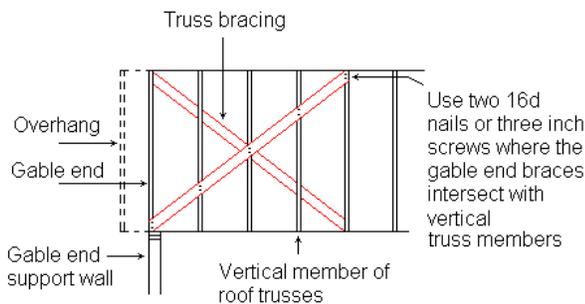
home, you need to do something else and the recommended method is to use a gable end brace. But remember that hurricane winds switch direction as they move through, so the North side could use this treatment as well.
