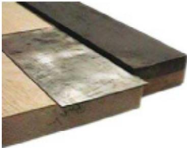
For more demanding scraping applications, such as finished work, you will need to smooth out the edges you just filed. The edge is smoothed on a bench sharpening stone. It is best to use the edge of the stone so you don't wear a groove in the top. The easiest way to smooth the edge of the scraper is to lay
